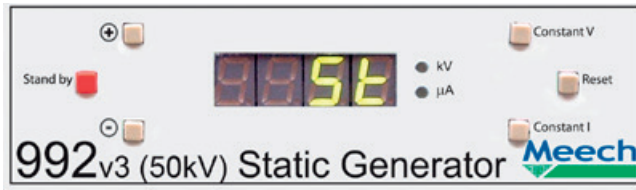
Display with 992v3-50kV in Stand by function
