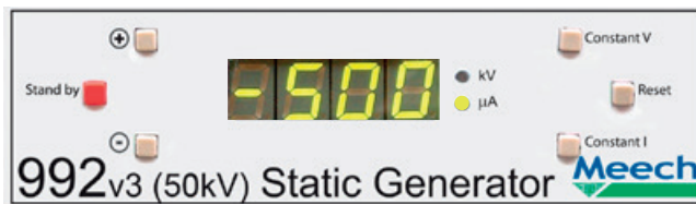
Display with 992v3-50kV operating in Constant Current Mode
