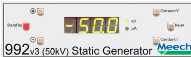
Display with 992v3 50kV operating in Constant Voltage Mode
