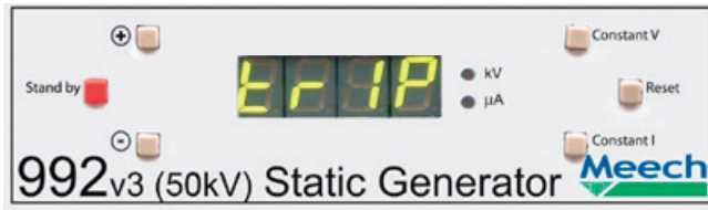
Display with 992v3-50kV “Tripped” out
